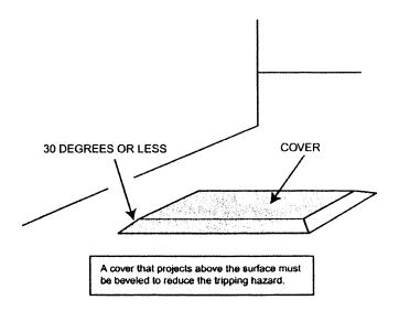
(2) You must prevent tools and materials from falling through a floor hole. The floor hole must be protected by a cover that leaves an opening no more than one inch wide and is securely held in place. This applies only to floor holes that persons cannot accidentally walk into on account of fixed machinery, equipment, or walls.
